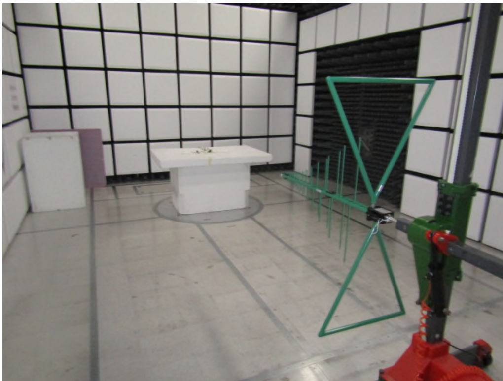
Figure 1: Radiated Emissions – Front – Below 1GHz
