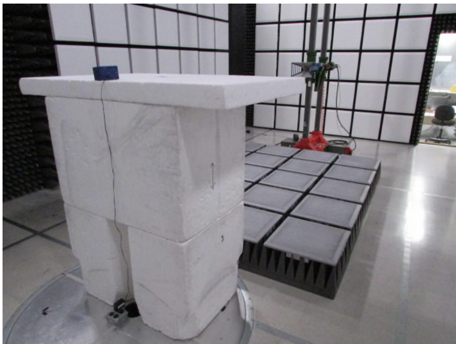
Figure 6: Radiated Emissions – Back – Above 1GHz
