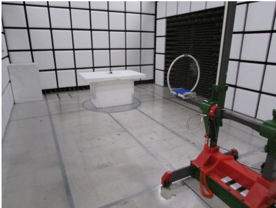
Figure 1: Radiated Emissions – Front – Below 30MHz
