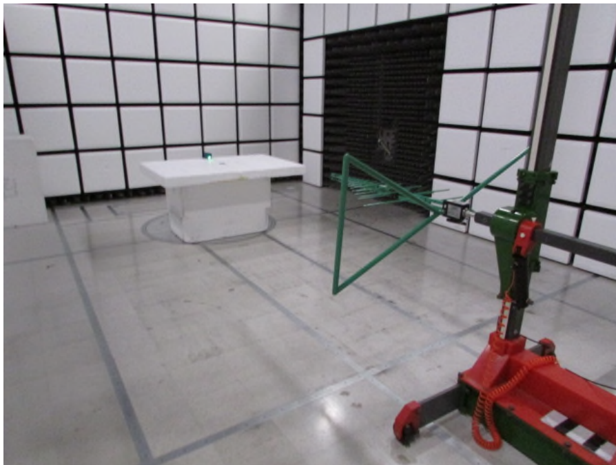
Figure 3: Radiated Emissions – Front – Below 1GHz
