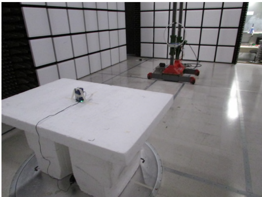
Figure 2: Radiated Emissions – Back – Below 30MHz
