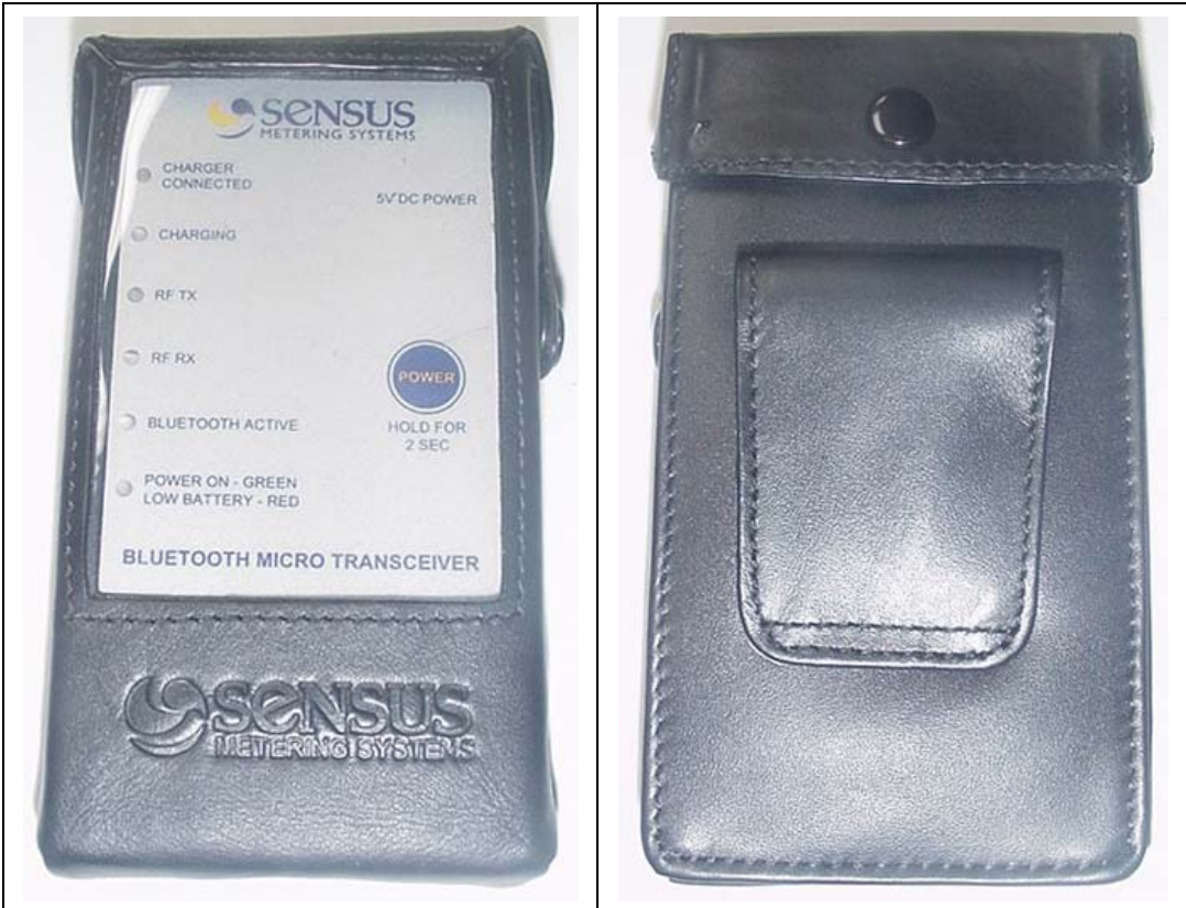
Front Side of DUT with Belt-worn Case Accessory Back Side of DUT with Belt-worn Case Accessory
