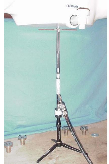
835 MHz Validation Dipole Setup
