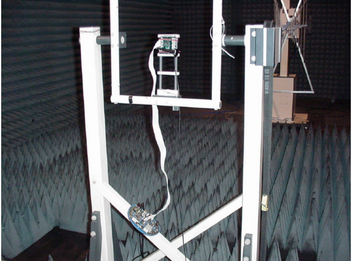
Photo 1: Test setup for radiated measurements (fully anechoic chamber, tests > 1 GHz)
