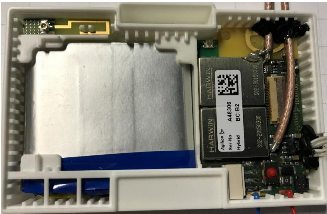
Photograph 4: : EUT B, front overview, battery inside
