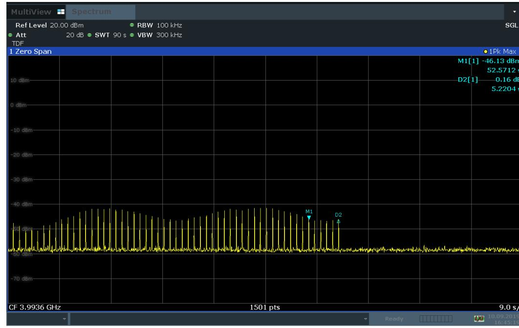
**1.4. Connection between EUT D and intentional radiator (AE7) is established. The door of the FAR is opened at first part of the measurement. EUT D is moved all the time. The door of the FAR is closed at time M1 (thereby the communication between EUT D and AE 7 is interrupted).**
