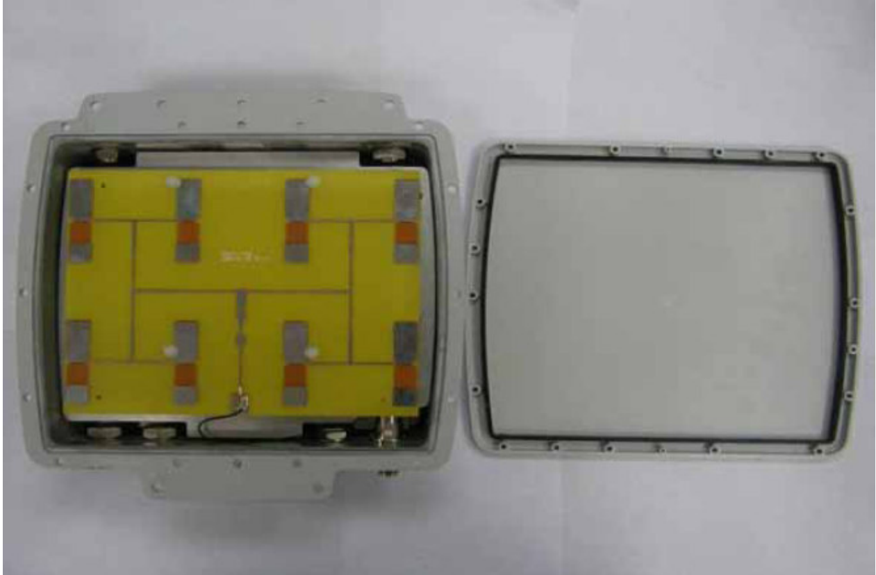
B. Internal Patch 2 Antenna (Antenna Gain : 11.29dBi)
