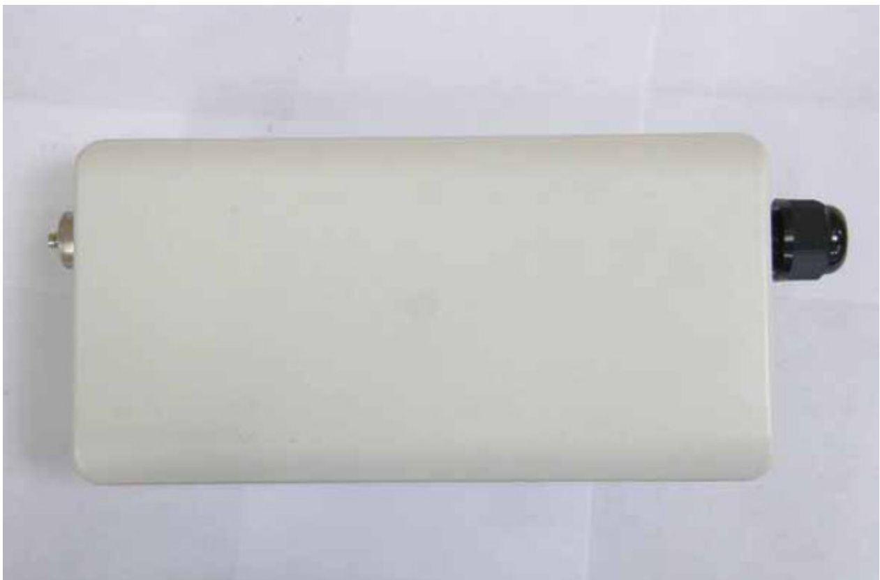
B. Internal Patch 2 Antenna (Antenna Gain : 11.29dBi)
