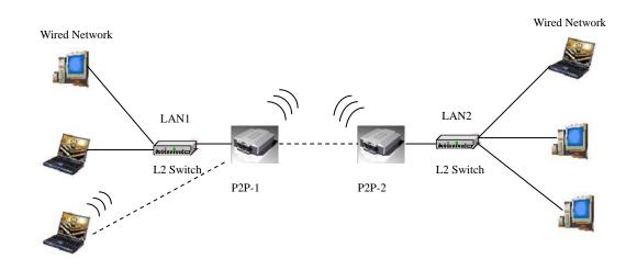
PtP mode setting is like AP mode setting, but encryption only WEP encryption method can select. When wireless0 or wireless1 in PtP mode will also do AP function, suggest disable SSID broadcast(Pull down select "y" in **hidden SSID** to disable SSID broadcast) and set WEP encryption.
