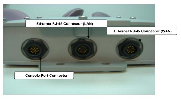
Console Port --- It is used for initial setup and configuration of the device
