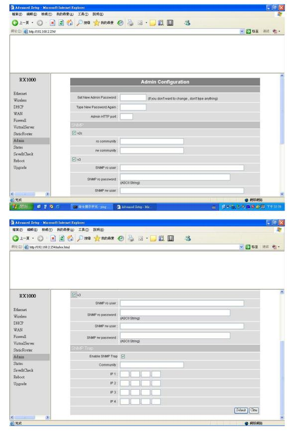
You can change login password (default password is "**default**"), SNMP user name and password, and SNMP Trap setting here.
