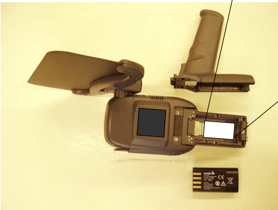
Picture 3: NordicID PL3000 pistol grip and battery removed
