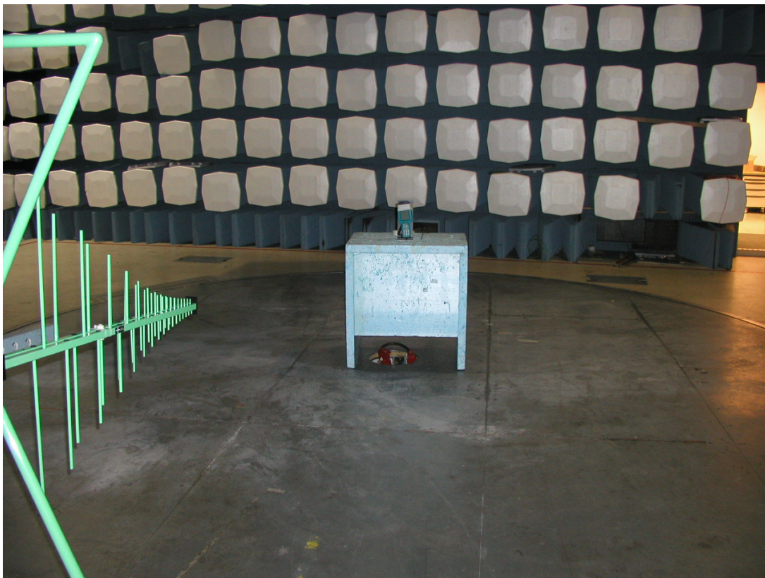
Photograph 2. Radiated emissions test setup.
