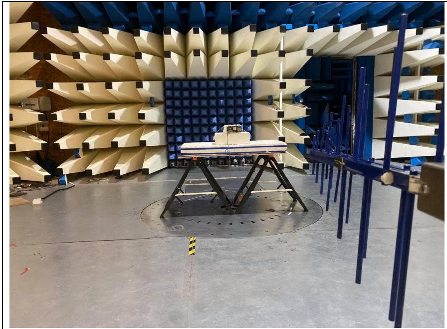
Fig 2 Test setup 300MHz -1GHz Rad Emissions
