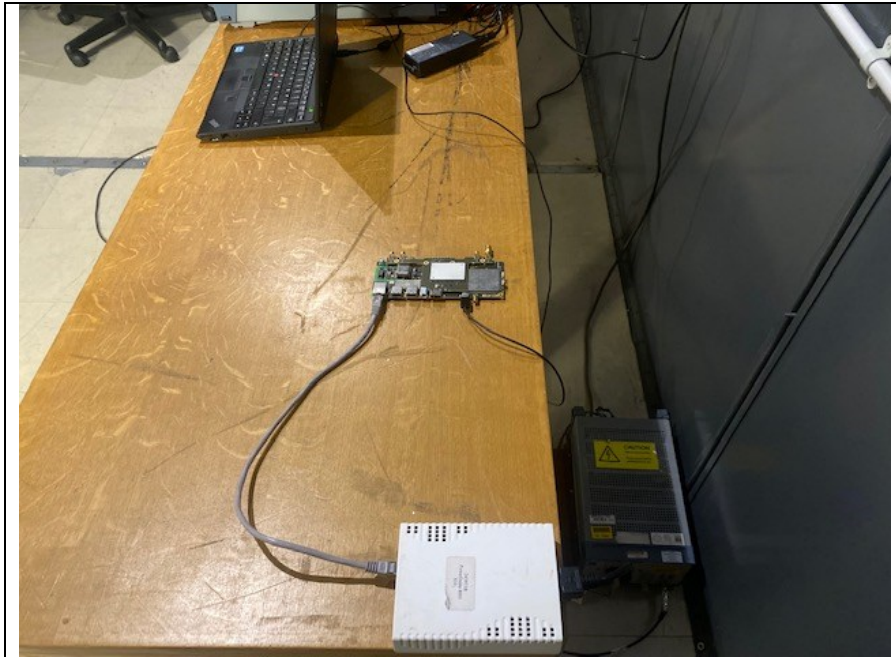
Fig 6a Test setup Conducted Emissions on the mains
