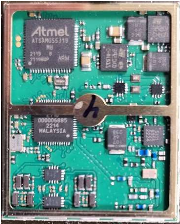
Picture 1. NUR3-1W module without shield
