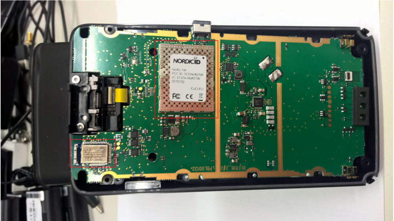
Pic. 4: EXA51e CPU board TOP view. NUR2-1W with RF shield and MBT42Q BLE module location.
