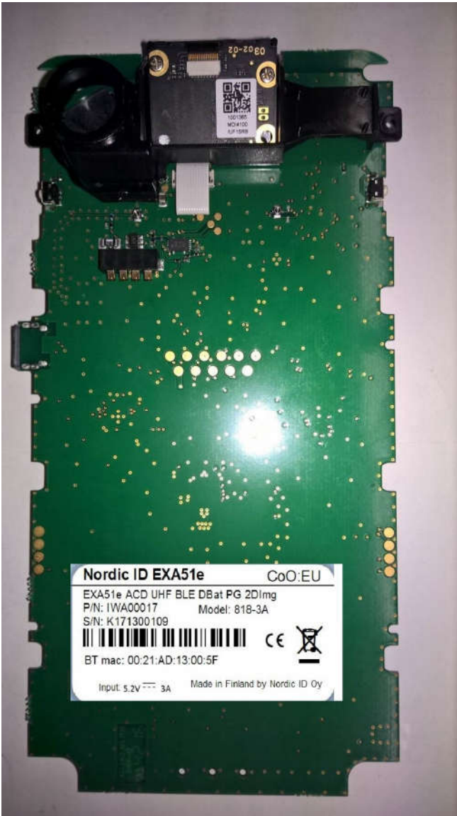
Pic.5:EXA51e CPU board bottom view with type label.
