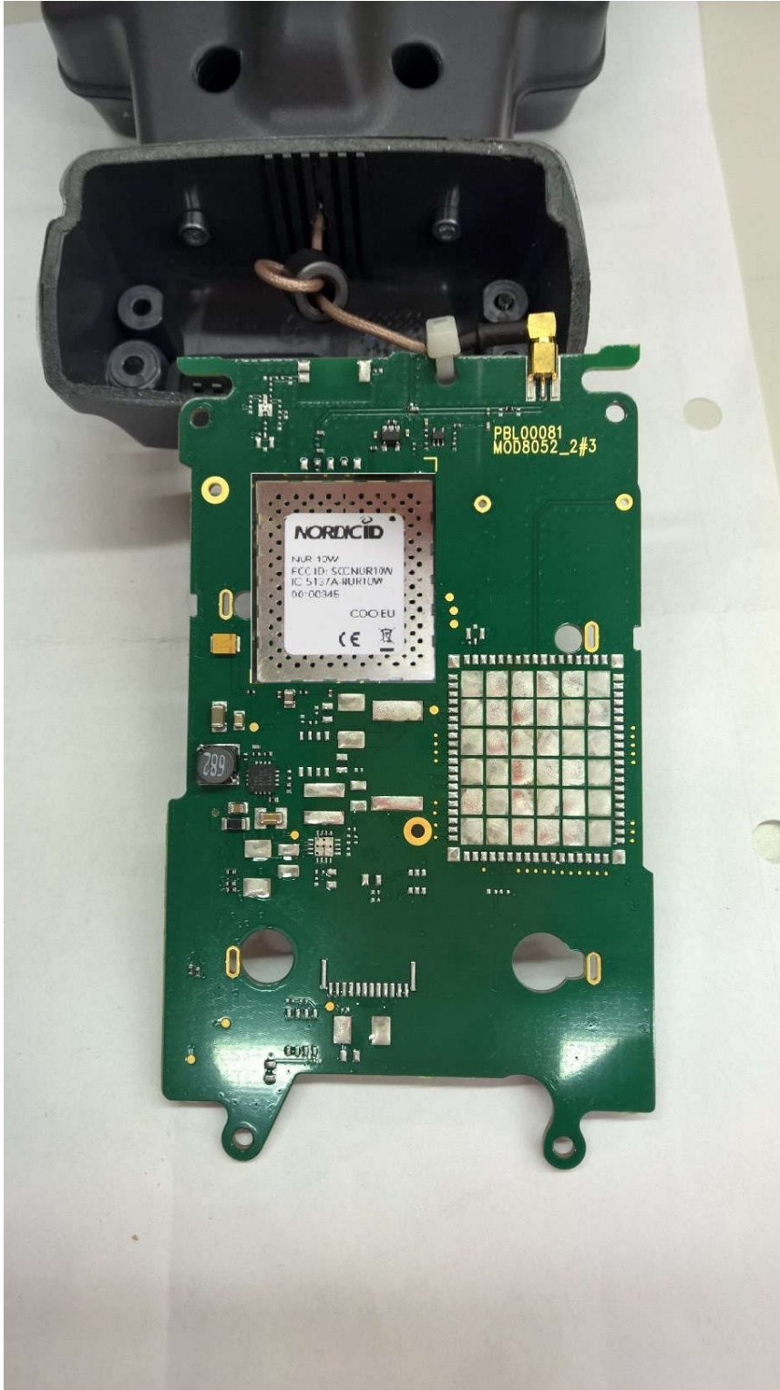
Picture 16. NUR-10W RFID module in Merlin CD ONE 805-2F Mod board (top view).
