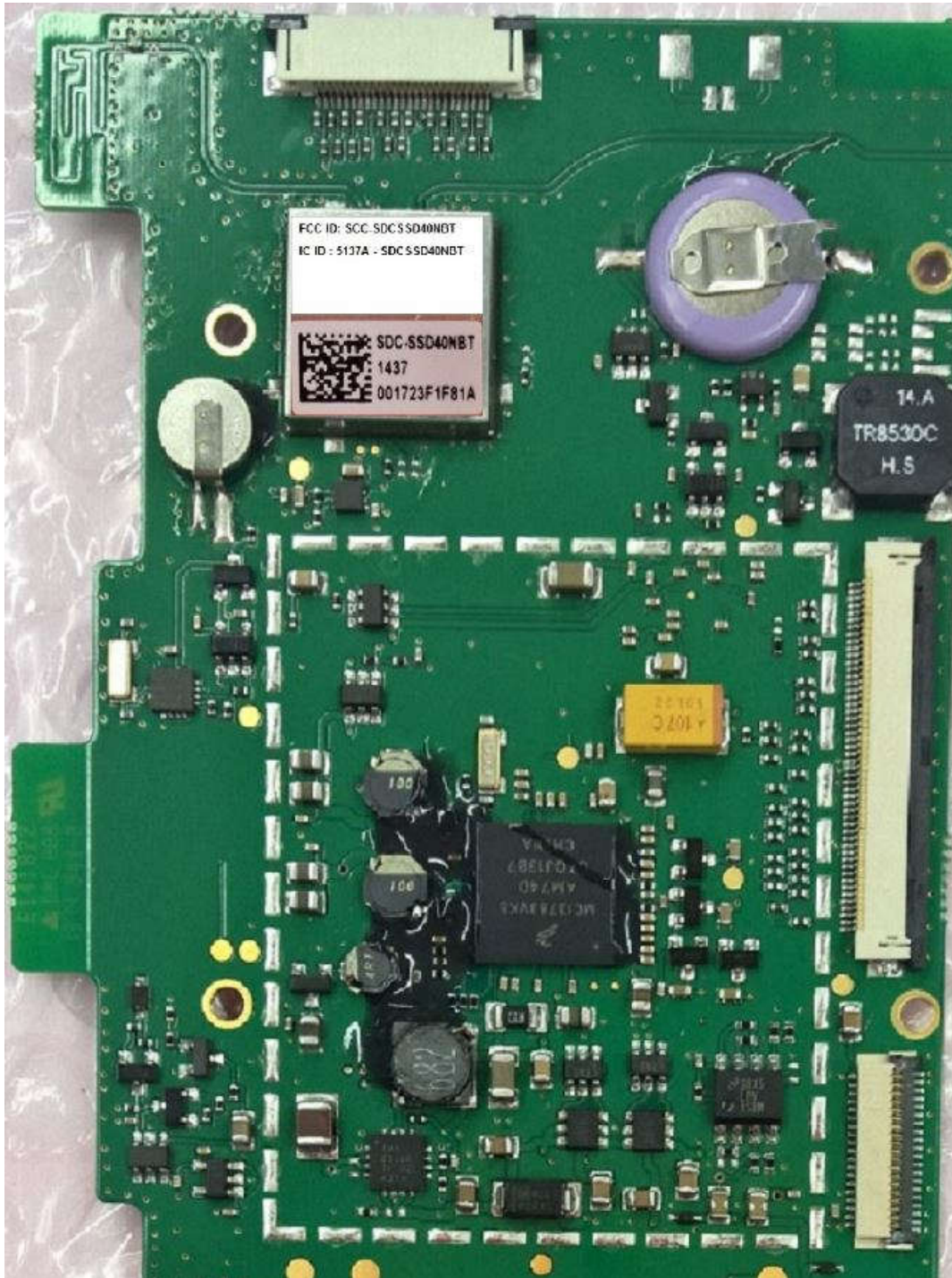
Picture 13. SDC-SSD40NBT module in Merlin CD 805-2A main board.
