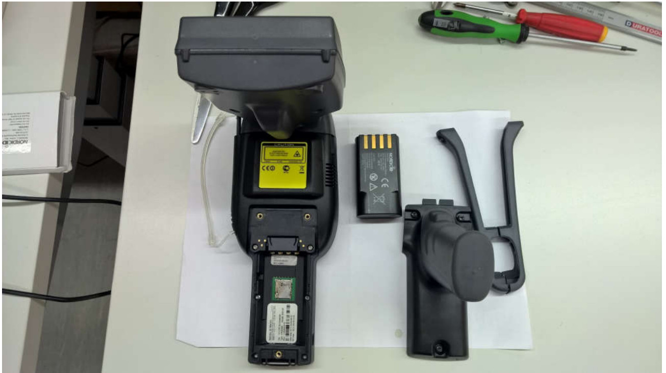
Picture 7. Merlin CD pistol grip and battery removed.
