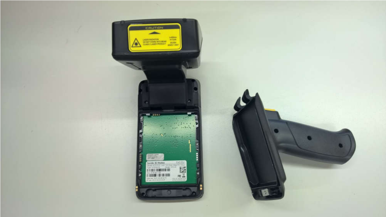
Picture 20: NordicID Medea ACD pistol grip detached / battery slot
