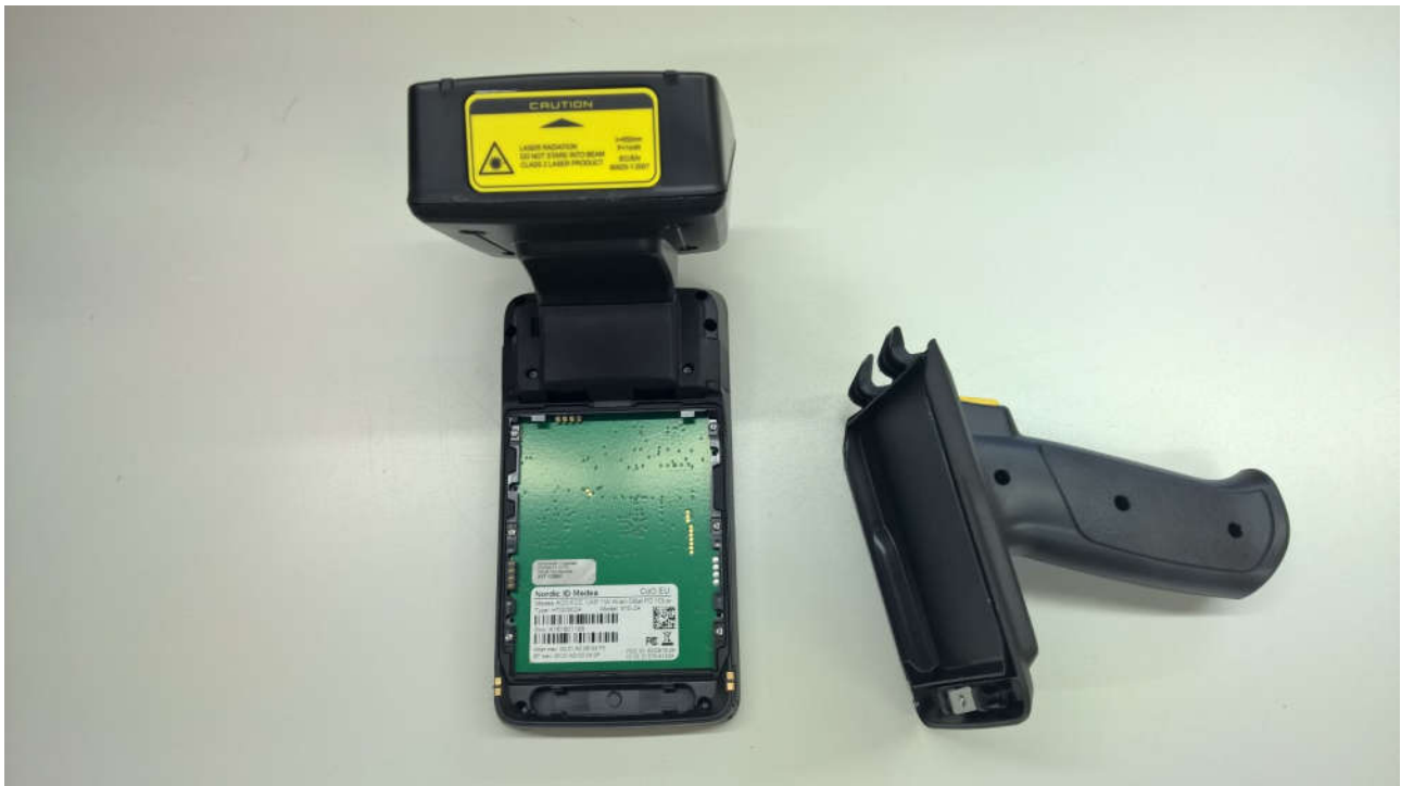
Picture 5: Medea ACD type label location under battery slot.
