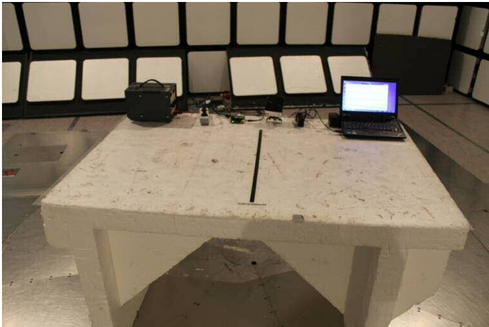
Photograph 2. The EUT and test set-up for radiated emission test.
