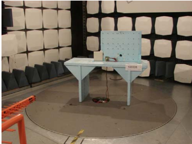
Picture 4: Transmitter Radiated emission test setup <1 GHz
