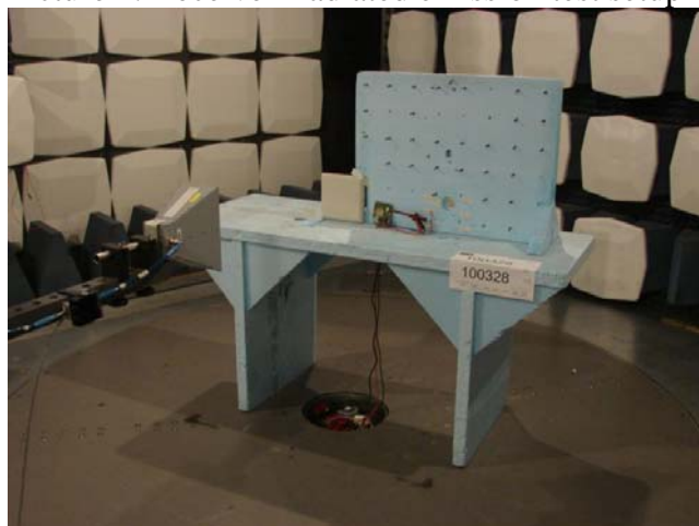
Picture 3: Receiver Radiated emission test setup 1 GHz – 5 GHz
