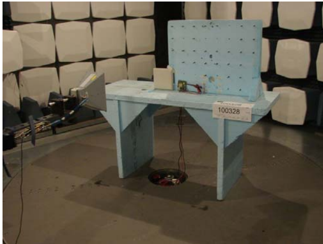
Picture 5: Transmitter Radiated emission test setup 1 GHz – 10 GHz.
