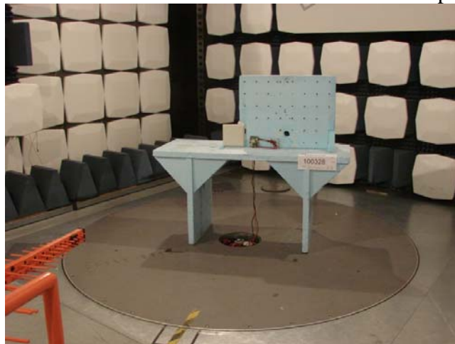
Picture 2: Receiver Radiated emission test setup <1 GHz
