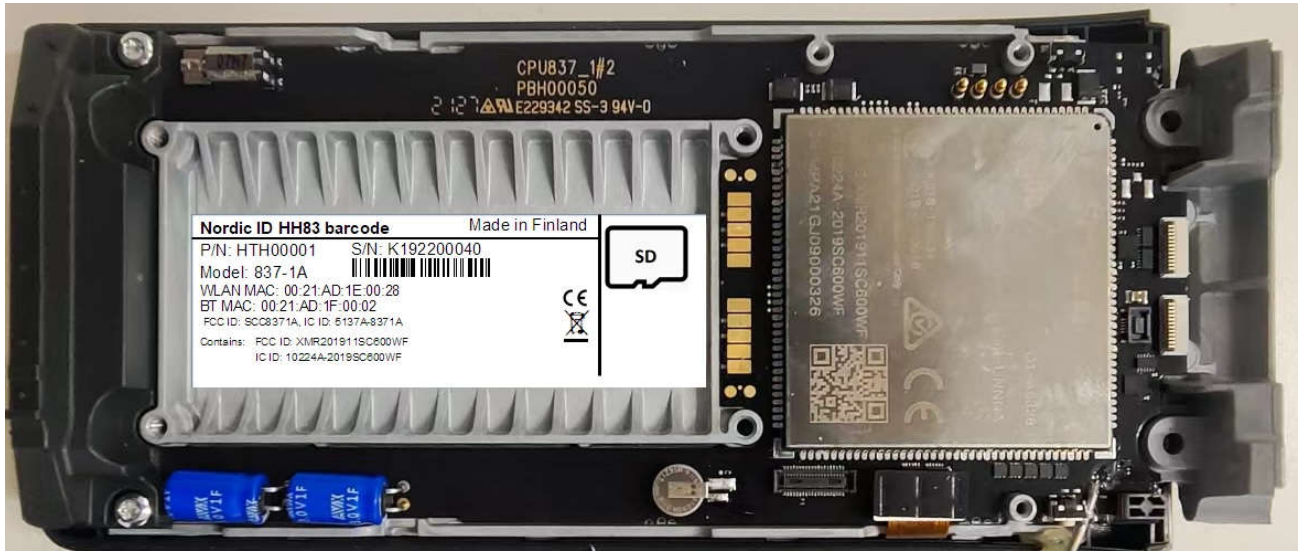
Picture 3. HH83 BARCODE main unit internal.
