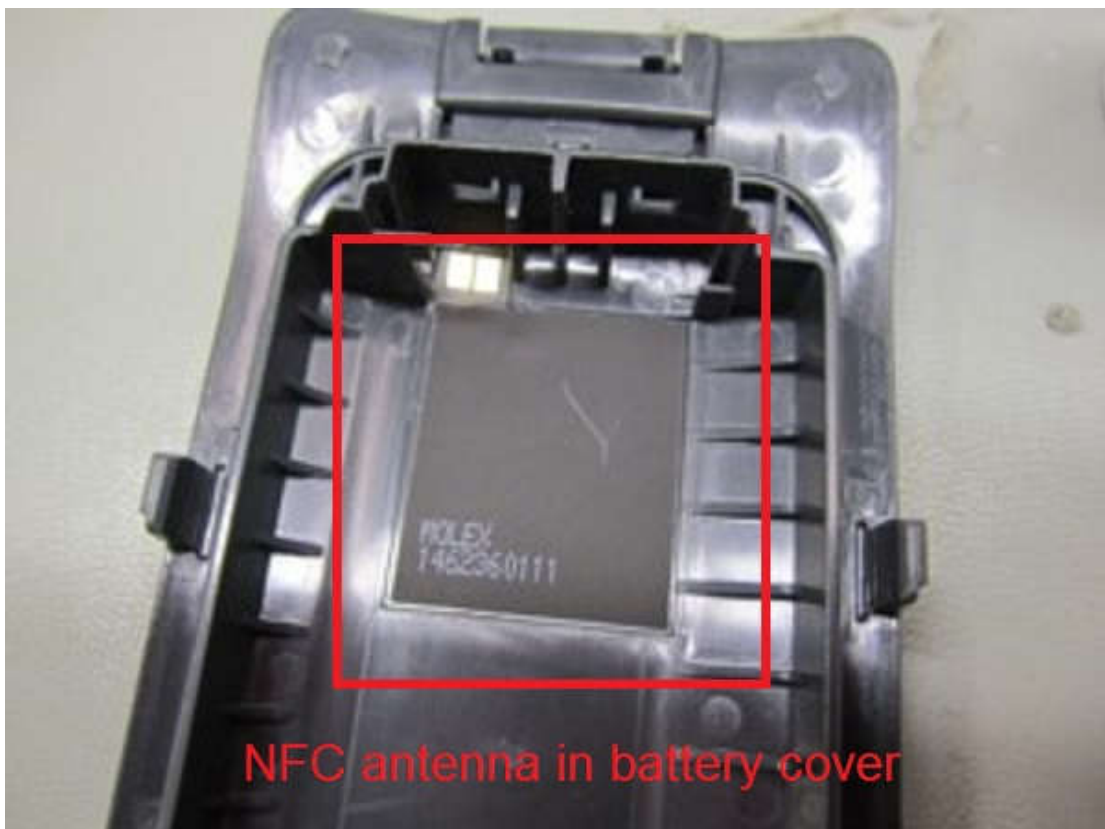
Picture 10. NFC antenna in battery cover.
