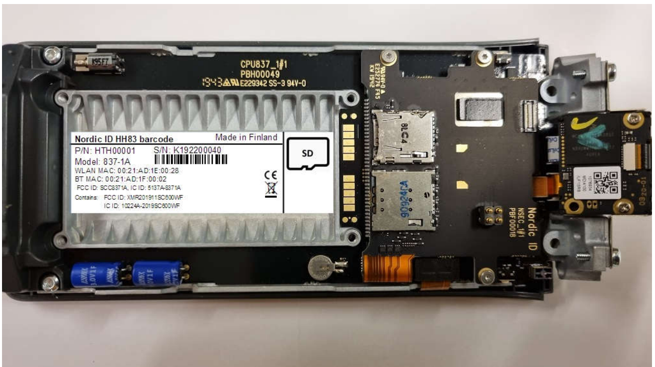
Picture 2. HH83 BARCODE main unit internal.
