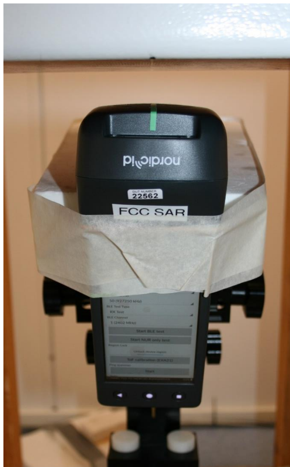
RFID reader's top side against the phantom with 20mm separation distance.
