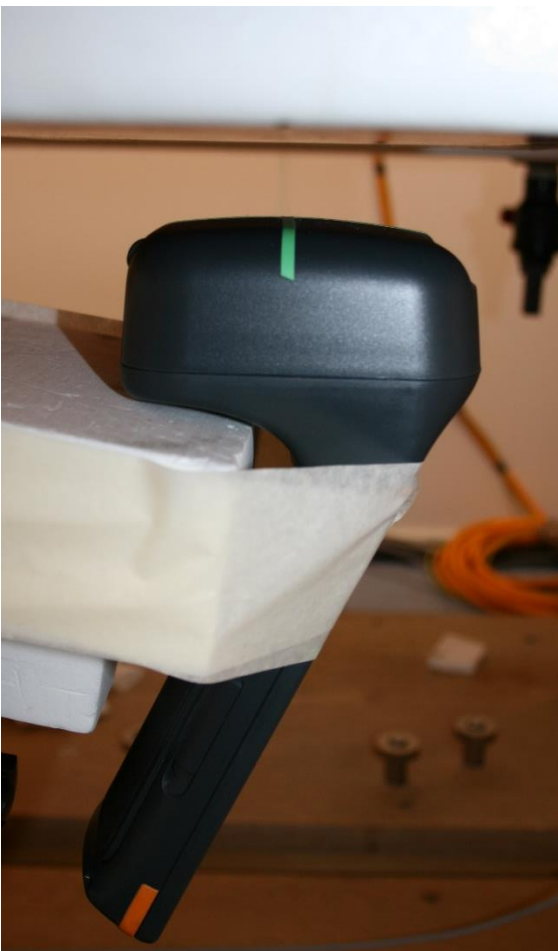
RFID reader's top side against the phantom with 20mm separation distance.
