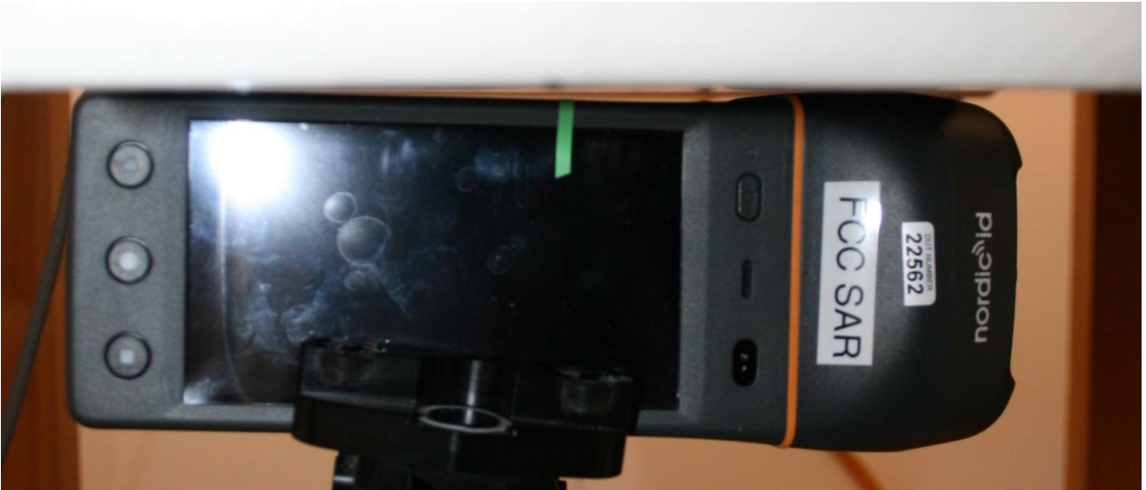
The left side of the device against the phantom with 0mm separation for WLAN testing
