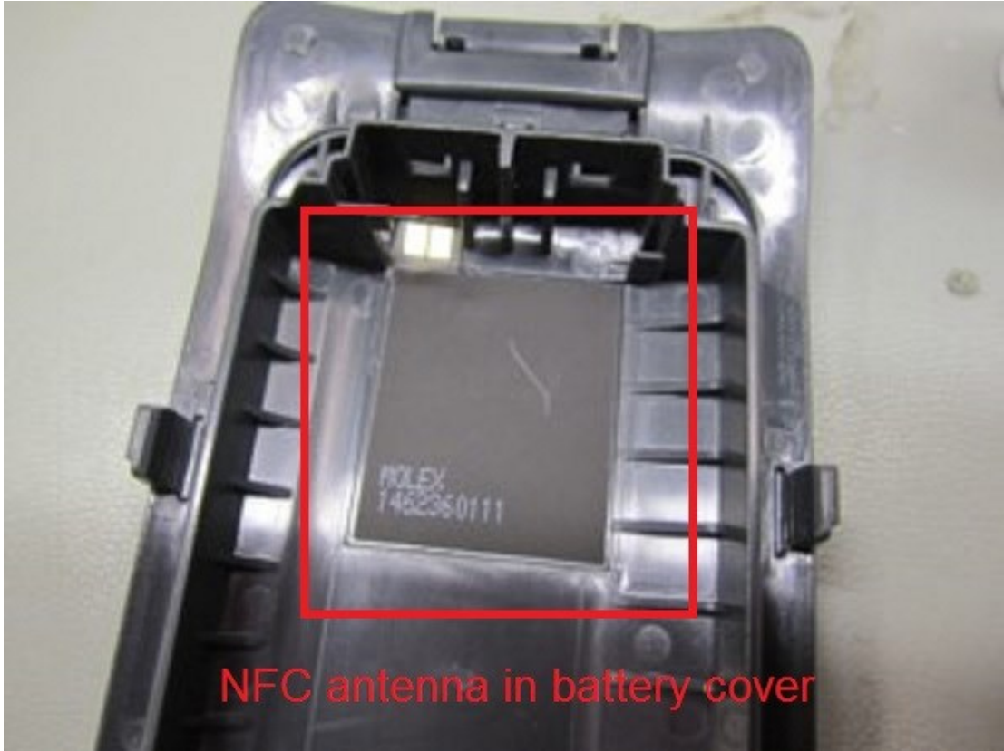
Pic 4. NFC antenna assembled into battery cover. Antenna is Molex 1462360111.
