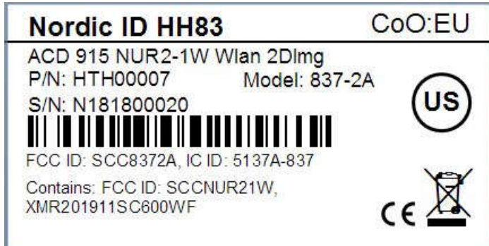
Pic. 1. HH83 UHF RFID ACD, Model 837-2A FCC&IC type label.
