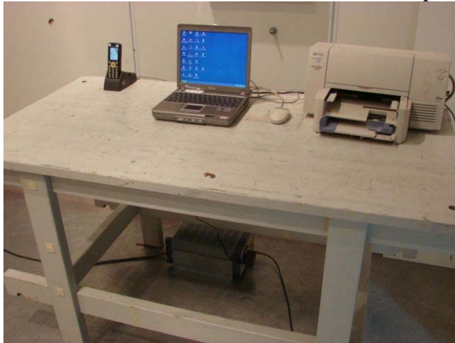
Picture 2: Conducted emission measurement test setup
