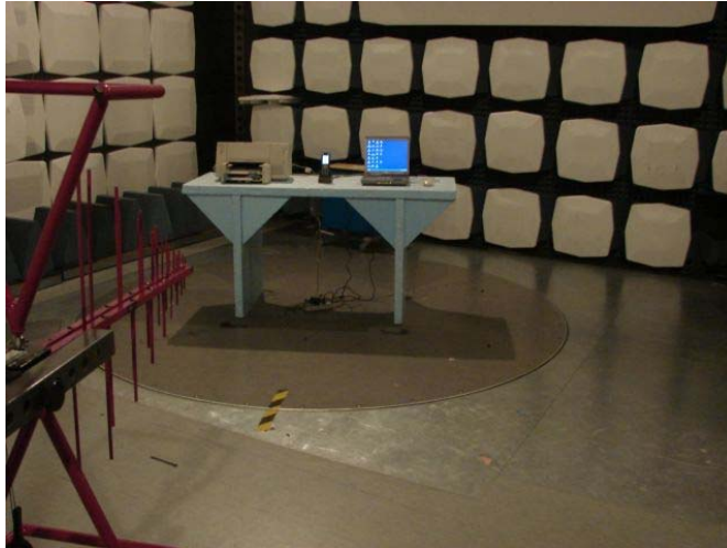
Picture 3: Receiver Radiated emission test setup <1 GHz
