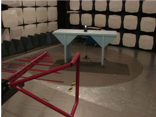
Picture 5: Transmitter Radiated emission test setup <3 GHz
