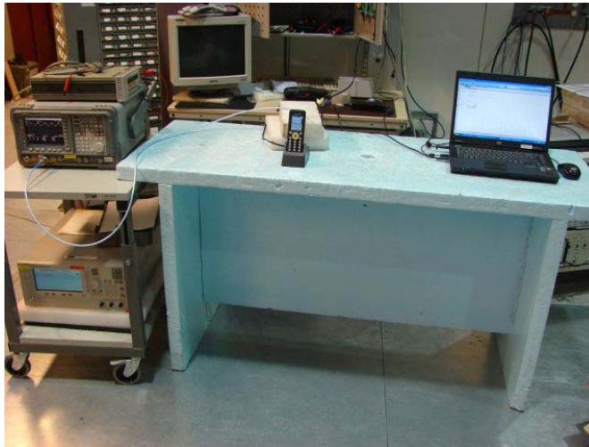
Picture 1: Conducted RF measurement test setup
