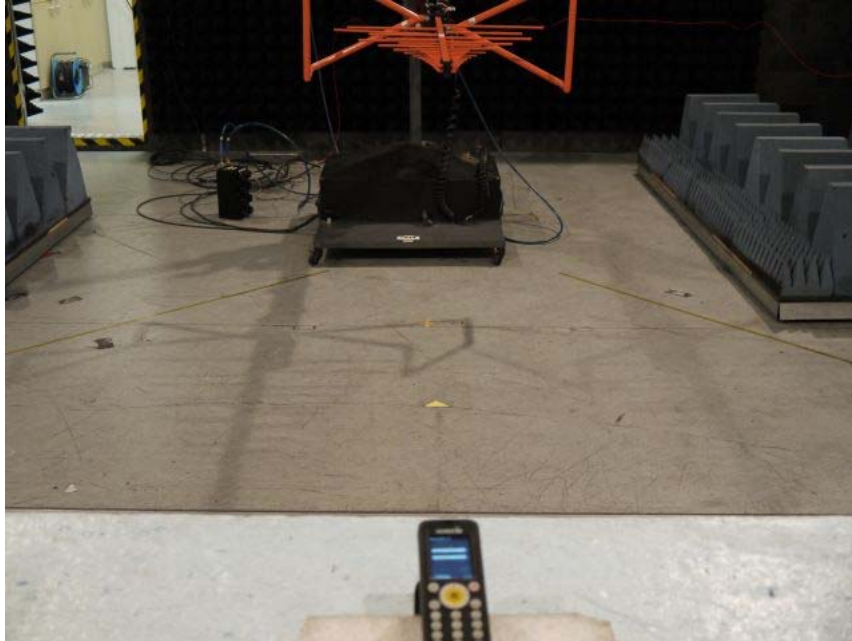
Picture 1: Radiated emission test setup 30 MHz – 1 GHz
