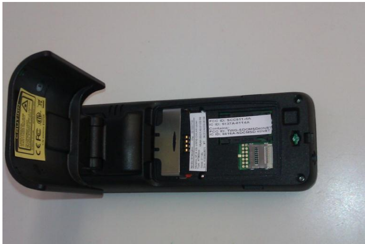
Picture 4. NordicID Morphic Hand Terminal with approval label, type label and FCC/IC ID label
