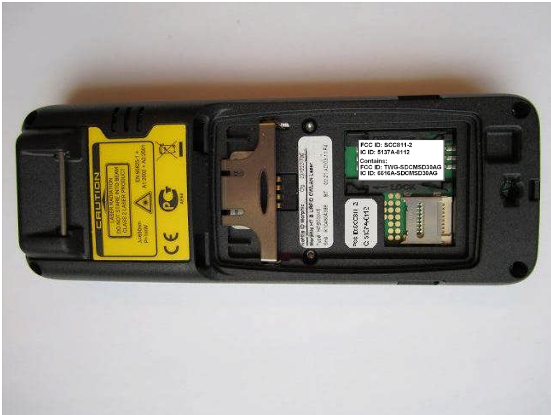
Picture 4. NordicID Morphic Hand Terminal with type label and FCC/IC ID label
