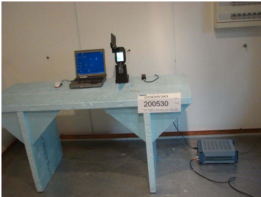
Picture 7: Test setup for measurement of conducted emissions to AC-mains
