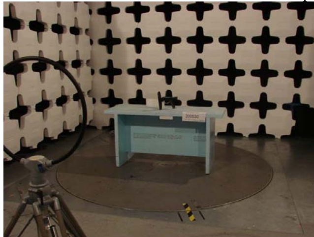
Picture 2: Radiated emission test setup 150 kHz – 30 MHz
