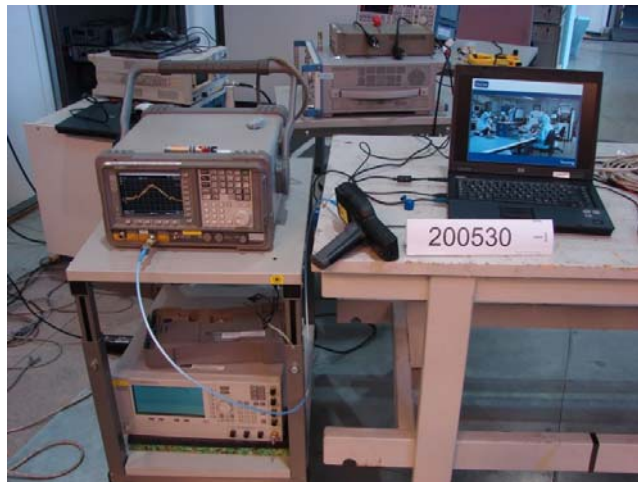
Picture 1: Conducted RF measurement test setup
