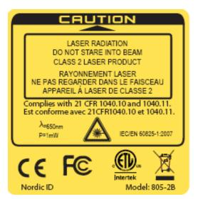
Nordic ID Merlin mobile computers, equipped with 1D laser scanner, are classified as Class 2 Laser products. The laser scanner uses the low power laser diode emitting visible light beam of 650nm wavelength with 1mW power. As with any very bright light source, such as the sun, the user should avoid staring directly into the light beam. Momentary exposure to a Class 2 laser is not known to be harmful.
