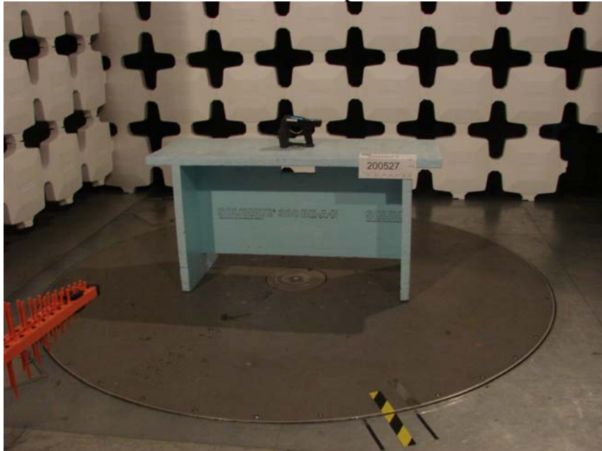
Picture 2: Radiated emission test setup 1 GHz – 16 GHz
