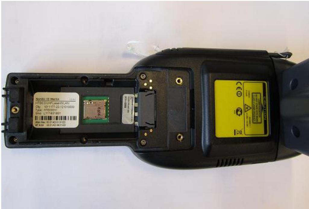
Picture 3. Nordic ID Merlin Hand Terminal with a type label
