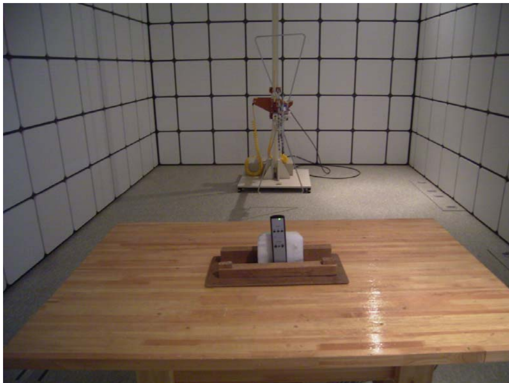
Radiated Emissions(30MHz~1000MHz)- Y View
