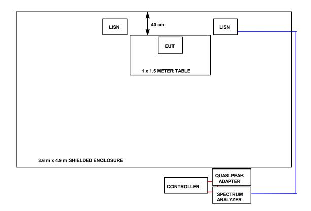
FIGURE 2: Radiated Emissions Test Setup
