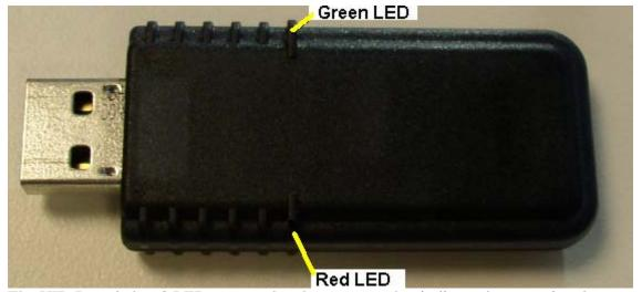
The HID Dongle has 2 LEDs, one red and one green, that indicate the operational states of the device. The red LED is used for binding and the green LED indicates data transfer from the HID device to the dongle.
