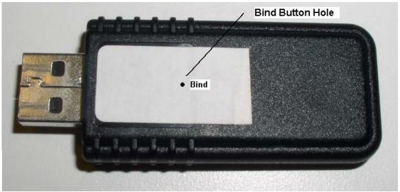
To use the HID Dongle, the user must first "bind" the dongle to the HID device (keyboard). This is typically done at the factory before shipment of the keyboard/dongle. However, the end user may also bind the device to a keyboard by pressing the "bind" button on the dongle, and on the keyboard. The dongle's bind button is internal to the dongle and must be pressed by inserting a paperclip or a small stiff wire into the bind button hole and depressing the button.
