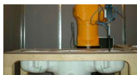
Figure 5.1 SAM Twin Phantom
