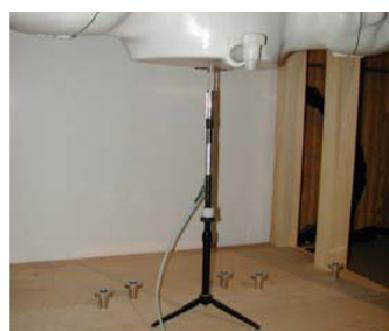
Figure 12.1 Dipole Validation Test Setup
