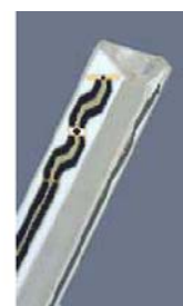
Figure 3.2 Probe Thick-Film Technique
