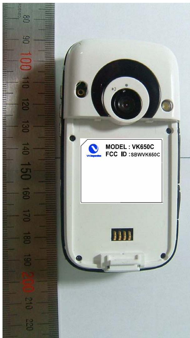
Note: 1. The label generally is located underneath a back door of the phone.
