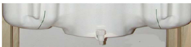
Figure 7.2 SAM Twin Phantom shell
