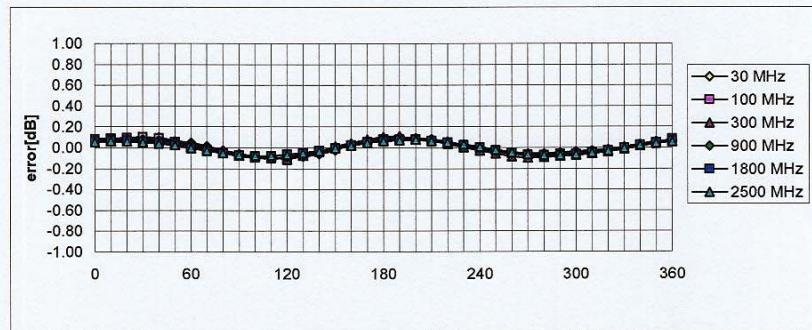
Axial Isotropy Error  $< \pm 0.2$  dB
