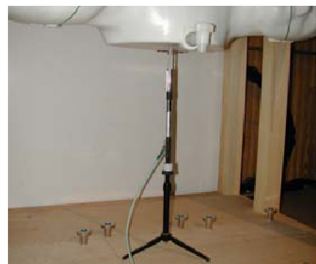
Figure 12.1 Dipole Validation Test Setup
