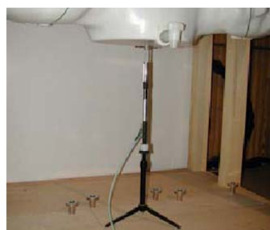
Figure 12.1 Dipole Validation Test Setup
