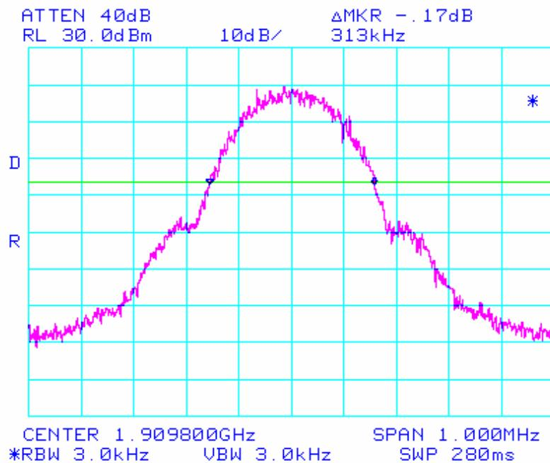
**GSM1900****Band Edge Ch. 512**
