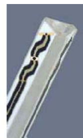
Figure 3.2 Probe Thick-Film Technique
