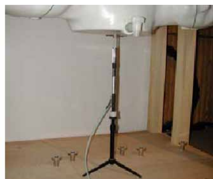
Figure 12.1 Dipole Validation Test Setup
