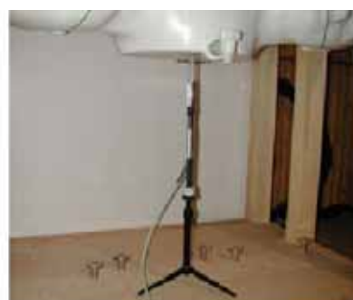
Figure 12.1 Dipole Validation Test Setup
