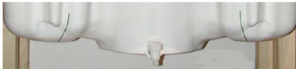
Figure 7.2 SAM Twin Phantom shell
