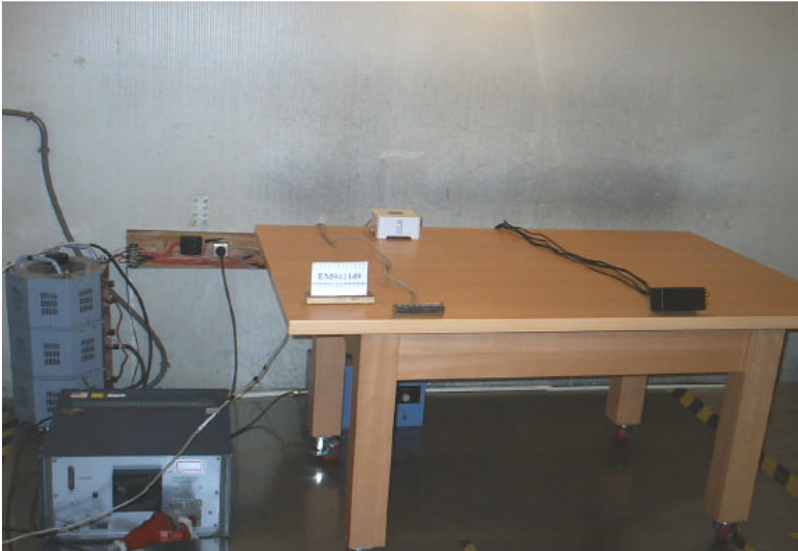
FRONT VIEW OF CONDUCTED MEASUREMENT
