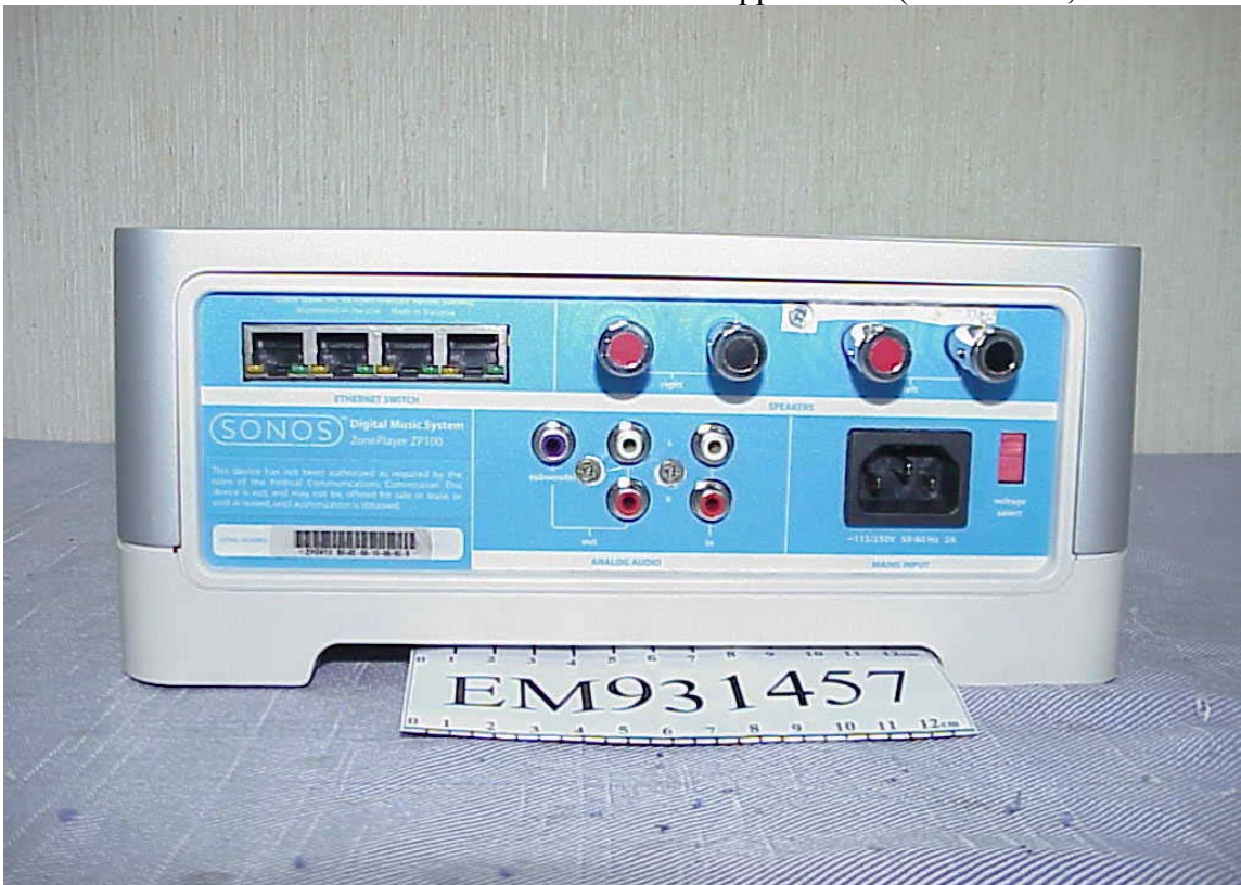
Figure 4 Appearance (Rear View, Interface Ports)
