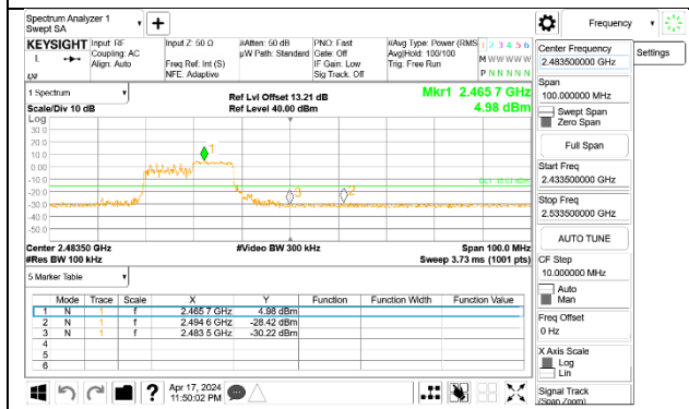
HIGH CHANNEL 11 BANDEDGE Antenna 3
