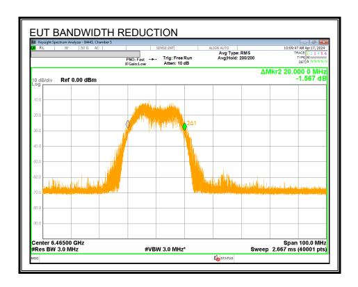
With the Incumbent Signal set to the Upper Edge f<sub>c3</sub> the EUT continues to operate at a reduced 40MHz bandwidth.
